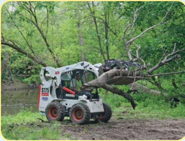
Figure 11 - If conditions allow, a small skid steer or tractor may be used to remove LWD
